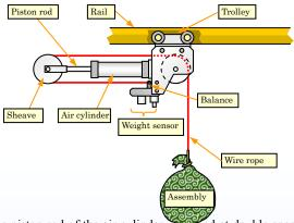
The piston rod of the air cylinder is moved at double speed with a sheave and the assembly is moved up and down with a wire rope.
