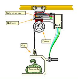
A wire rope take-up spool rotates through the ball screw in the air cylinder with the large diameter mounted into the drum to move the assembly up and down.
