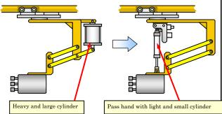
For the pass hand, the cylinder is directly moved with the less operation force, therefore, there is no need to depend on a conventional double speed mechanism.
