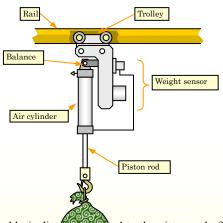
The assembly is dire Assembly ted to the piston rod of the air cylinder for the up and erations.
